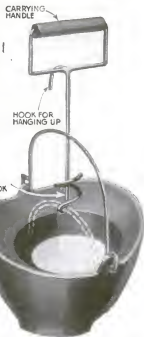
This safety-first pot-hook is designed to prevent burns from overturned solder-pots
