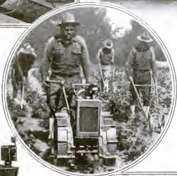
Operated in small spaces this baby tractor was adopted by the government for work in camp gardens. It plows or cultivates, runs a washing machine, pumps water, in fact does a variety of odd jobs
