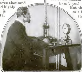
In testing the surface hardness of metals a hard steel ball is forced against the metal by hydraulic pressure. This man is watching the manometer indicating the pressure applied in the test
