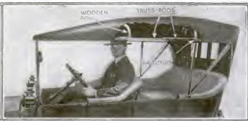
This contrivance attached to the Ford top converts it into a one-man design which can be raised or lowered at will. How clean-cut this is compared with the car at the left
