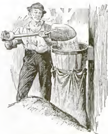
With this arrangement for holding the sack, one man can do the work of two in filling
