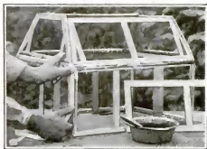
The framework sections are fastened together with carpenter's glue and tape
