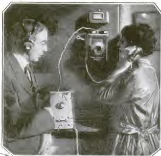
Hooked up with the wired telephone lines and with the antenna post of the radio receiving set, as shown in wiring diagram at left, the adapter converts the telephone wires into a wireless aerial without interfering with telephone conversations
