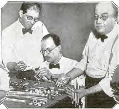
Blown from half-inch glass tubes, artificial eyes are "painted" by fusing colored glass into them. At left: Shaping an eye before a blowtorch. At right: Cutting a glass tube, that later will become an artificial eye.
