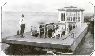
Above is shown the barge, equipped with sounding and recording mechanism used by government engineers in making profile maps of the river bed along the upper Mississippi. The operation of the machine is shown at left. Note the vanes that steady the lower end of sounding arm on the river bottom.
