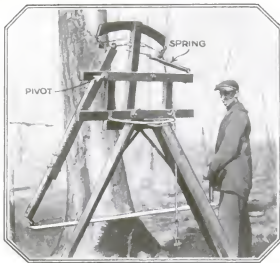
One man can work this saw; he pulls on his end and a spring jerks the saw back
