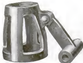
A grip has been invented that fits over the muzzle end of a riveting hammer and has a projecting handle that the riveter grasps; his work is thus made much easier
