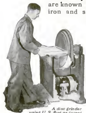
A disc grinder using U. S. flint or garnet paper smooths wooden things up in a jiffy. Disc grinders are made in various sizes; horizontal and vertical types.
