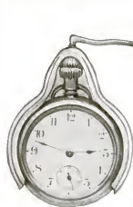
This mechanical watch-winder saves many sore fingers in a large repair shop
