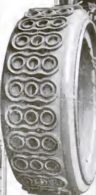
These metal pads encircle the tires and prevent slipping without the usual unpleasant bumping. The holes in the pads increase the traction
