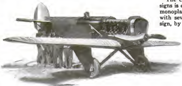
The powerful new Loening racing monoplane, showing how the engine is supported by the heavy braced monoplane wings. Note the comparatively short length of the light fuselage
