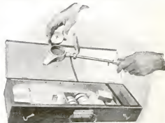
A combustible briquet, inserted into soldering iron, supplies the heat
