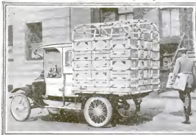
Here is a truck body made from gas-piping. The rear doors are also of pipes, which slide into each other when opened. The novelty of the scheme should appeal to truck-owners
