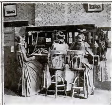
This is an actual photograph of one of the first crude multiple switchboards, showing "central" operators at work. These instruments, the forerunners of our modern switchboards, connected only a few hundred telephone subscribers
