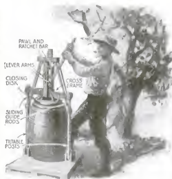
After the barrel has been placed in position on the base of the machine, the downward motion of a lever will press the head of the barrel home into its groove
