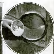
A combination lamp and reflector forms a unit that fits into the headlight socket without interfering with the dimmer
