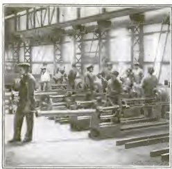
Hot iron is poured into these machines and whirled into pipes by revolving molds
