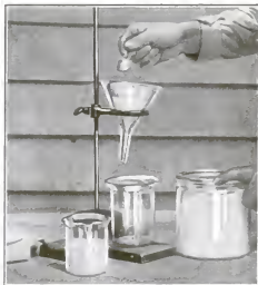
Here is the way to separate oil from water. A funnel, filter paper and a container are all that is necessary.
