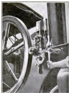
Small Gas Engine "Cranks" Large Road Roller
