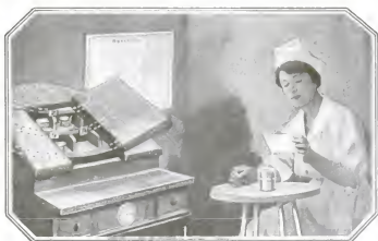
When the clock strikes, a door flies open and a bottle of medicine stands behind it on a revolving table; there is a table for each hour of the day
