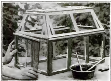
Face pieces similar to the main frames are glued on to complete the glass covers
