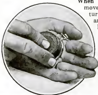
Refractory watch-cases yield to this form of persuasion in short order. A vacuum cup affords a good grip
