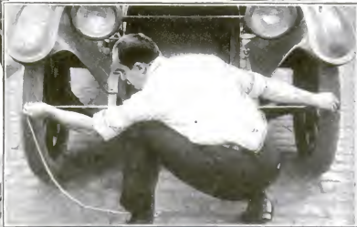
One simple way to determine whether your front wheels are in alignment, and so prevent excessive tire wear. Measure the distances between the centers of the tires at the front and the rear. Besides being in alignment, the wheels should "toe in"—that is, they should be closer together at the bottom than at the top
