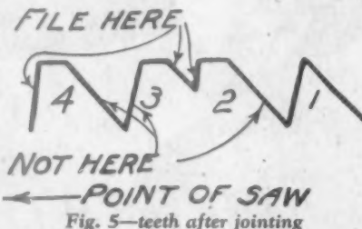
Fig. 5—teeth after jointing
