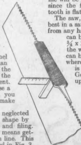
Fig. 3—jointing a saw
