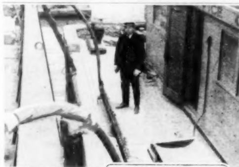
On Each Side of the Barge Is a Manifold with 20 One-Inch Hose Connections
