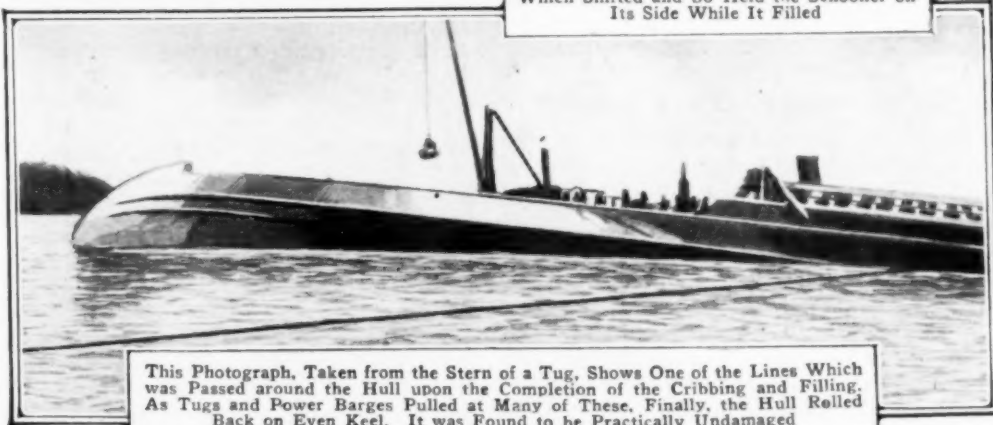
The Building and Filling of the Third Row Brought the Schooner to Approximately the Position Pictured. On the Deck can be Distinguished the Remains of the Deck Load, Which Shifted and So Held the Schooner on Its Side While It Filled
