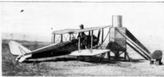
The Local Oil Merchant Delivers the Drums of Gasoline to the Top of the Tower, Seen at the Right, and So Makes an Airdrome Pumping Outfit Unnecessary. The Plane is being "Gassed," at the Left
