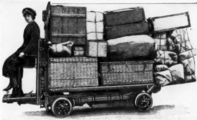
The New Electrical Truck is Characterized Chiefly by the Fact That the Motor, Battery Container, and Other Parts, Are Independently Removable Units. This Makes for Quick Repair and Minimum Loss of Operating Time
