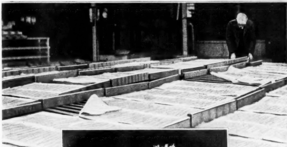
The Drying Tables upon Which the Agar is Spread after Bleaching
