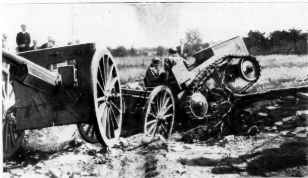
The Three-Ton Tractor, Designed to Take the Place of Horses for Hauling Field Ordnance, Surmounts Obstacles with Extraordinary Agility, Thanks to the Peculiar Spring Suspension of Its Idler Wheels
