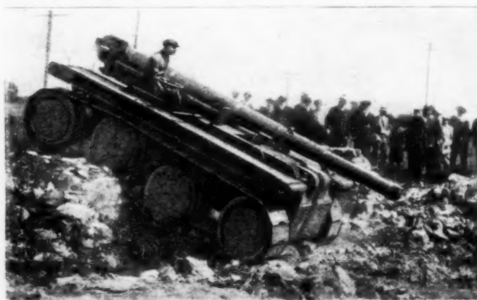
The Eight Large Wheels Which Distinguish the Mount of the Six-Inch Gun Make the Endless Tread Highly Effective in Climbing over Obstacles. The Weight of the Outfit Complete Is Only 22 Tons
