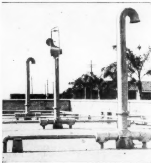
Practical Ventilator Test: Two Gooseneck Devices Are Visible, While between Them can be Seen One Equipped with a Revolving Hood
