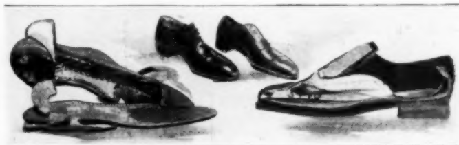
The Two Shoes in the Background have been Dissected to Show the Differences in Construction. At the Left Is the Part-Paper Shoe, at the Right, the All-Leather Article
