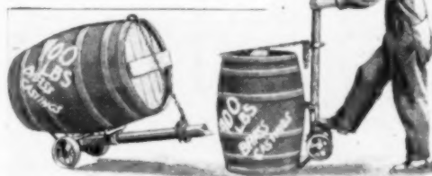
The Worker is Preparing to Tilt the Load Back over the Wheels. The Load is Carried as Pictured at the Left
