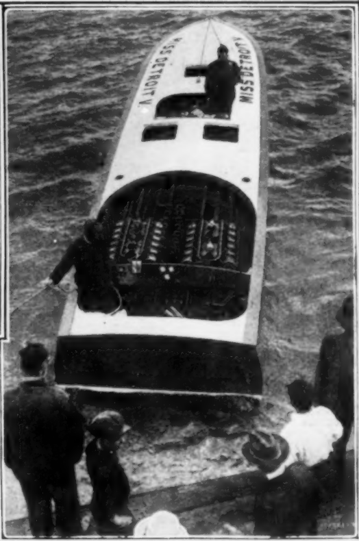
The "Miss Detroit V," Pictured at the Right, and in Stern View, Above, Was Third in the First Race, but in the Second Recovered Itself, and Crossed the Line Only Half a Minute behind the Winning "Miss America." Both are Equipped with Two 12-Cylinder Marine Engines Aggregating 840 Horsepower
