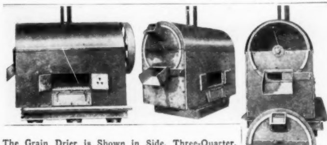
The Grain Drier is Shown in Side, Three-Quarter, and Front Views. A Part of the Front has been Removed, at the Right, to Show the Interior of the Iron Cylinder. At the Left is Seen the Grate for the Fire of Coal, Wood, or Corncoals
