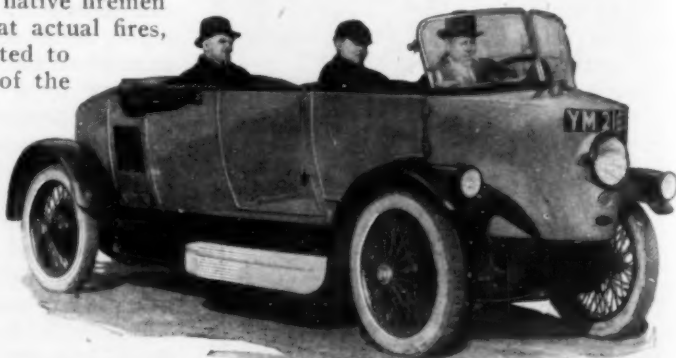
Engine Heat Does Not Bother the Driver of This German Car, For Motor Is Placed at the Rear
