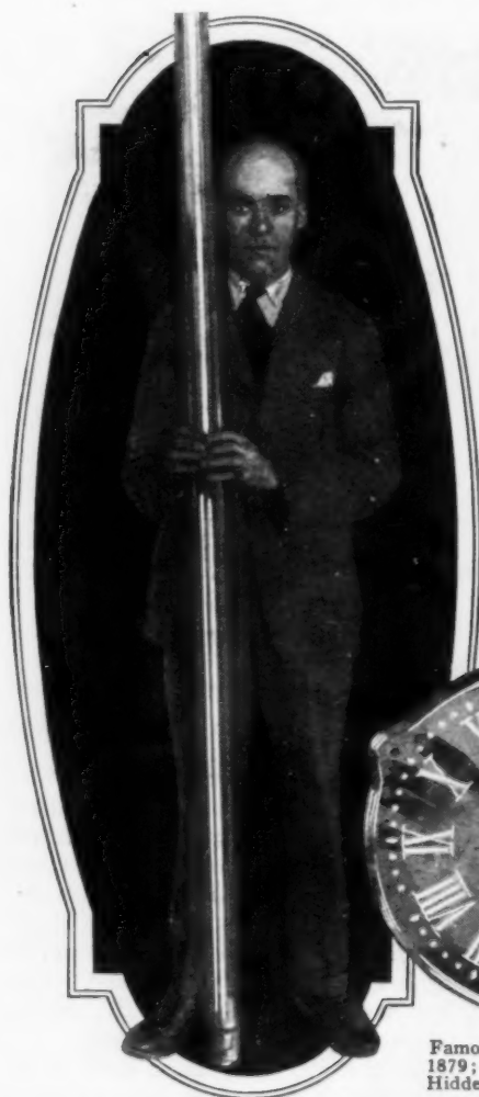
One of the First Vacuum Tubes Invented; It Is Seven Feet Long
