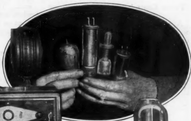
New Tube with Parts; It Uses 110-Volt Alternating Current and, Having No Filament, It Cannot Be Burned Out
