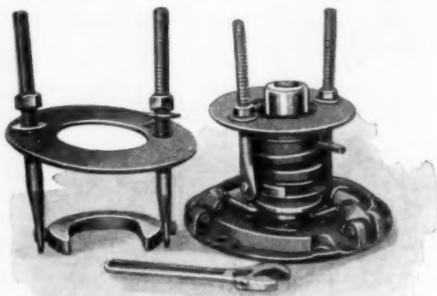
Spring Compressor for Ford Clutch. Simplifies Task of Removing Spring
