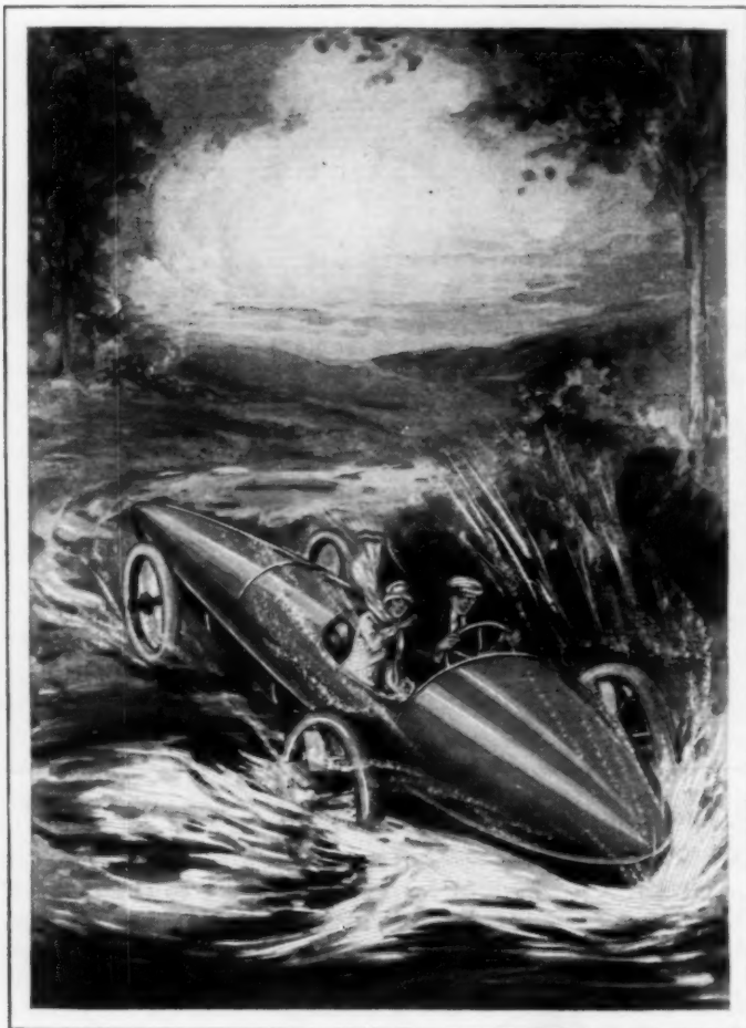
When Auto Is Driven into Deep Water, Paddles on Front Wheels Propel the Car like a Boat
