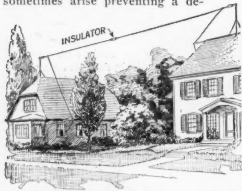
Divided Aerial Showing the Position of the Insulator Midway between the Two Houses
