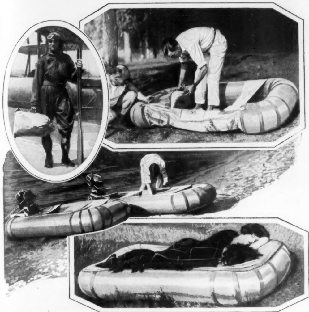
Lieut. Comm. Byrd with Boat in Bag: Blowing It Up by Sections for Use: Two with Outboard Motors, and in Service as a Bed; When Used for Latter Purpose, Canvas on Bottom Keeps Out Cold
