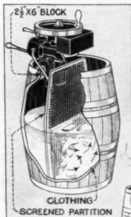
Outboard Motor Fitted on Barrel Is a Good Substitute for Washing Machine
