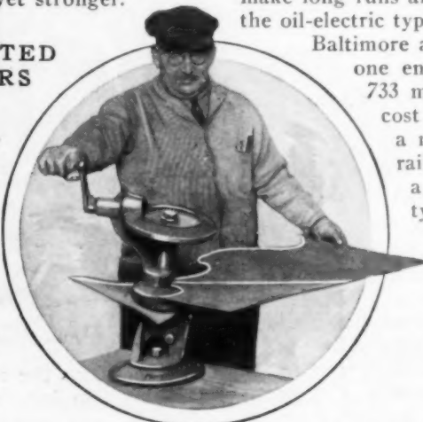
Metal Cutter in Operation: Curved or Irregular Pieces Are Easily Sheared Out
