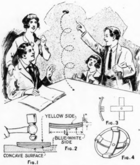
Toy Flipper Easily Made of Thermostatic Metal Amuses Everyone
